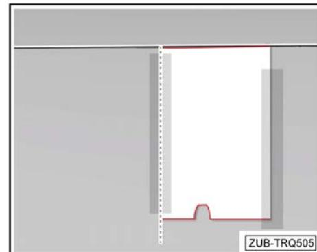
**-4- Remove the protective paper from the anti-glare film -1-. Position the anti-glare film -1- on the inside of the windscreen using the template and carefully press it on.**
